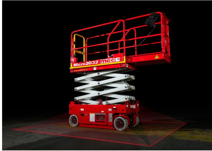
MEC's Perimeter Laser Lighting solves the challenge of dropped object risk by projecting a precise laser pattern onto the floor, clearly marking a warning zone around an active scissor lift. This laser solution offers great adjustability, superior quality, and performance creating a distinct, thin, long line safety perimeter around the machine. On floors with load limits, the lights outline the area outside the machine without overlapping, enhancing safety for load leveling.
