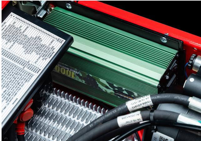
MEC's 1000W Inverter provides on board AC power at the platform for power tools and lithium power pack charging while avoiding the risks and limitations of overhanging power cords.
