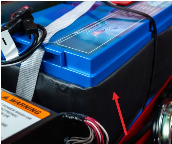
MEC's Cold Weather Package is designed to boost performance in low temperatures and includes a battery blanket for slab scissor machines and lighter viscosity hydraulic oil. It's effective in environments as cold as 0°F. For usage in even lower temperatures, please consult the factory.
