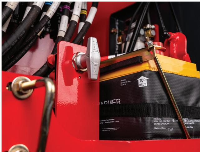
The battery disconnect switch cuts power from the battery to the electrical system, helping to prevent electrical drain during storage and ensuring safety during maintenance. The switch can also be locked in place for added security.
