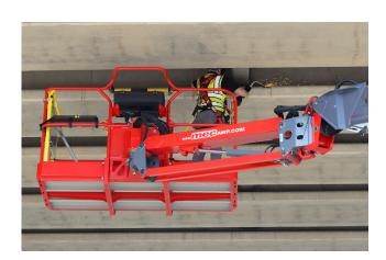
As part of MEC's MAX Series, the 66-RJ is built to lift more—without compromising reach or control. It supports up to 900 lbs of capacity at full height or out to 50 ft of outreach. Even at its maximum 56 ft outreach, the 66-RJ delivers an **industry-best unrestricted capacity of 600 lbs for a rotating jib boom.** This performance gives crews the strength to carry tools, materials, and multiple operators exactly where they're needed.
