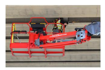
As part of MEC's MAX Series, the 66-RJ is built to lift more—without compromising reach or control. It supports up to 900 lb of capacity at full height or out to 50 ft of outreach. Even at its maximum 56 ft outreach, the 66-RJ delivers an **industry-best unrestricted capacity of 600 lb for a rotating jib boom.** This performance gives crews the strength to carry tools, materials, and multiple operators exactly where they're needed.
