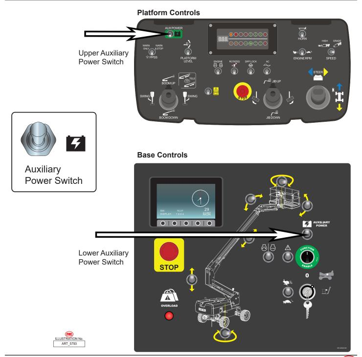
The Auxiliary Power System is used to lower the platform in case of primary power failure. To lower the platform, activate the Auxiliary Power Switch to run the auxiliary hydraulic pump.
