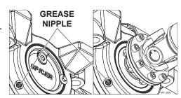
**Note:** Lubricate during service cycles.
