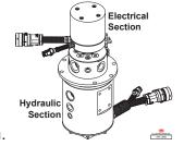
The Rotary Coupling connects electrical wires and hydraulic oil hoses between the chassis and the boom, so that the turret can rotate 360° without interruption.
