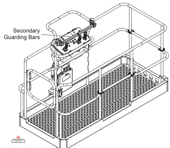
4. To enable limited operation while one or both bars are depressed, push up and hold the Emergency Platform Bypass switch (see illustration to right). While holding the Bypass switch, select the desired function and operate it in the normal procedure. Certain lift functions such as Riser Boom Up, Main Boom Up, and Telescope out are not available in this bypass mode.
