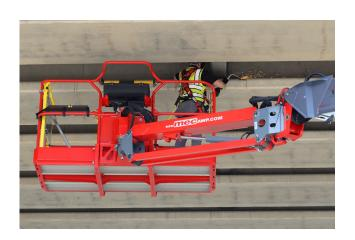
As part of MEC's MAX Series, the 66-RJ is built to lift more—without compromising reach or control. It supports up to 900 lbs of capacity at full height or out to 70 ft of outreach. Even at its maximum 80 ft outreach, the 66-RJ delivers an **industry-best unrestricted capacity of 600 lbs for a rotating jib boom.** This performance gives crews the strength to carry tools, materials, and multiple operators exactly where they're needed.
