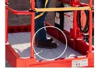
No foot switch allowing for greater mobility and comfort for the operator.
