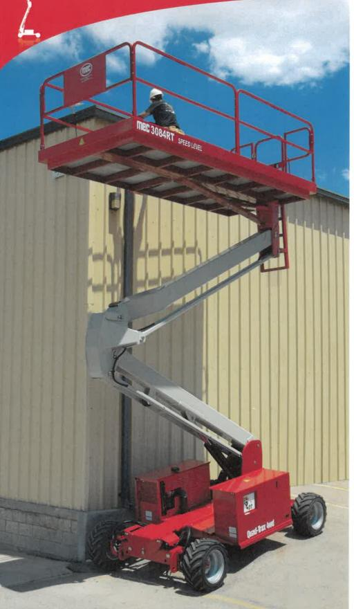
Unique Sigma Lift Design to Drive on Planar Slopes While Being Fully Elevated
