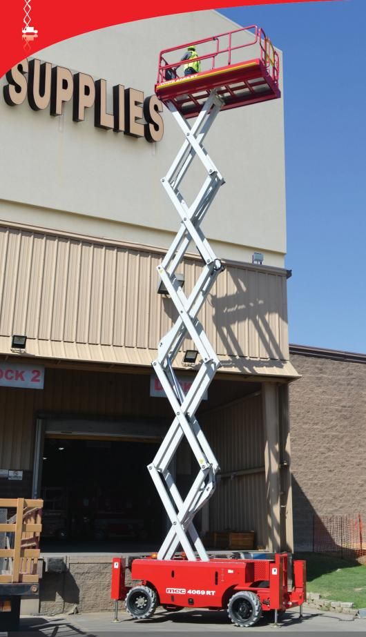
Flexible Platform Load Options Including Sheet Material Rack
