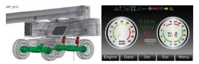
• In other cases, the oscillating axle of the machine is in a lock state, and the axle cannot oscillate to ensure the safety of the machine.
