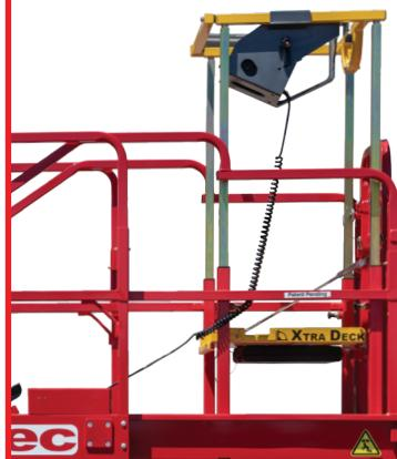
MEC's patented Xtra-Deck® can be deployed in less than 10 seconds.
