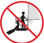
Check path before moving for crushing hazards when holding the platform rail.
