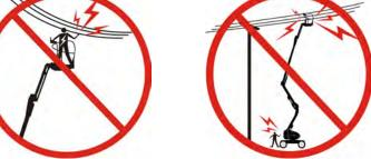
Maintain distance from electrical lines, apparatus, or any energized (exposed or insulated) parts according to the Minimum Approach Distance
