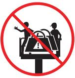
DO NOT exceed the maximum platform capacity. The weight of options and accessories will reduce the rated platform capacity and must be factored into the total platform load. Refer to the decals on the options or contact MEC.
