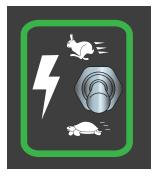
Press and hold this switch to enable and operate machine functions from the base controls.
