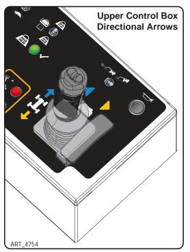
Depending on the orientation of the boom and chassis, the Drive and Steer functions may move the machine in directions opposite of the motion of the control lever. The color- and shape-coded arrows on the control lever decal correspond to similar arrow decals on the machine chassis (see illustrations). Be sure to check the arrows on the chassis before activating and using the Drive or Steer functions.
