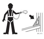
Personal fall protection equipment (PFPE) is required when operating this machine. All PFPE must comply with employer and job site rules and applicable governmental regulations, and must be inspected and used in accordance with the PFPE manufacturer's instructions.
