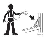
Personal fall protection equipment (PFPE) is required when operating this machine. All PFPE must comply with employer and job site rules and applicable governmental regulations, and must be inspected and used in accordance with the PFPE manufacturer's instructions.
