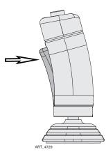
**Note:** If any Function Enable trigger or button is depressed for seven (7) seconds without any function being activated, the Enable System times out and deactivates. Release the trigger or button and reengage to activate the Function Enable System.
