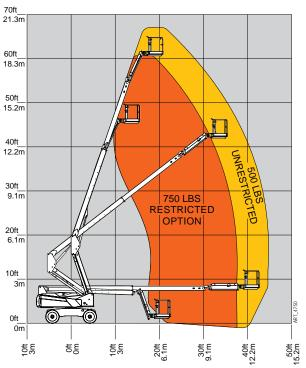
\*Working Height adds 6 feet (2 m) to platform height.
