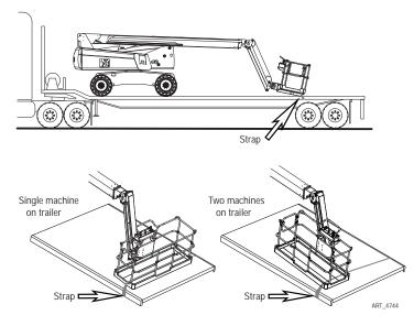
With the boom completely stowed, raise the jib slightly, then use the Platform Level function to lower the platform until the front of the platform touches the trailer surface.
