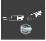
Move this switch to the left for high speed drive. Push this switch to the right for high torque drive.
