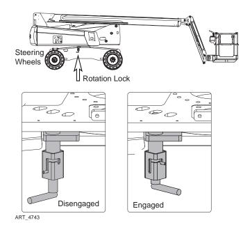
Before transport, rotate the turntable so that one of the three locking holes aligns with the Rotation Lock located on the chassis. The lock holes are located on the bottom of the Controls Module. The Rotation Lock is located on the chassis behind the left front wheel.
