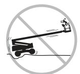
DO NOT DRIVE ON UNEVEN OR UNSTABLE SURFACE WHEN THE PLATFORM IS ELEVATED OR EXTENDED
