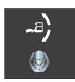
The platform will automatically level as the boom is lifted or lowered. The Platform Level function allows manual level adjustment of the platform. Manual leveling may be used to adjust the platform within 5° of level.
