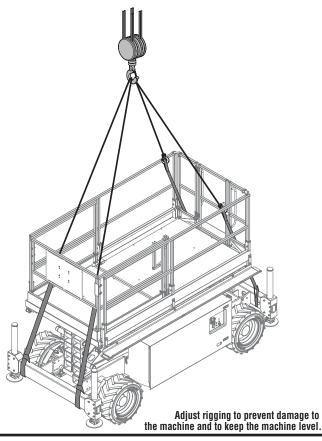
Fully lower the platform. Be sure the deck extension is retracted and the module doors are closed and secure. Remove all loose items from the machine.
