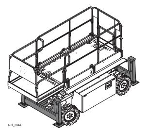
Lower the outriggers only when the machine is on a firm surface. The surface must be capable of supporting the maximum ground pressure per wheel/outrigger (see Specifications).
