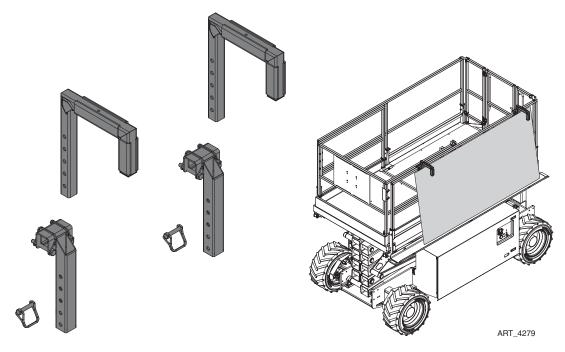
Remove the J-shaped arms from the Material Clamps when loading material on the Sheet Material Rack.
