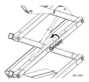
To set the Maintenance Lock, raise the platform enough to allow the Maintenance Lock to rotate to vertical. Carefully lower the platform until the pin above rests securely on the Maintenance Lock.
