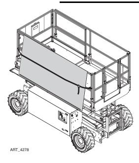
This machine is equipped with a Sheet Materials Rack. Up to 300 lbs (136 kg) of sheet material may be secured outside the platform to this rack. Maximum size of material on the Sheet Material Rack is 4' x 8' (1.2 m x 2.4 m) for outdoor wind loading. All material should be centered on the Sheet Materials Rack.
