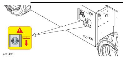
The Emergency Lowering System is used to lower the platform in case of power failure.
