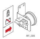
• Check Emergency Stop Switches at both the base and platform controls – turn clockwise to reset.
