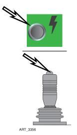
Lift functions (all boom, platform, chassis level and outrigger operations) are enabled by pressing and holding the button on top of either the Boom or Platform control levers, or the green Enable button at the top left of the Platform Control Station. This allows the use of multiple boom and platform functions if desired.
