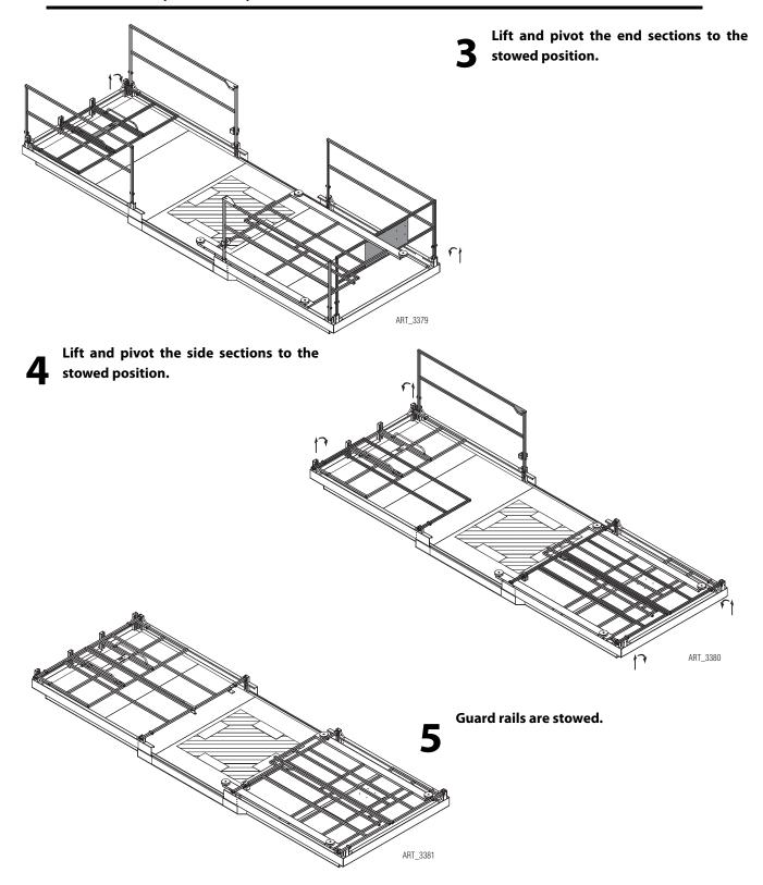
To return the machine to normal operation mode:
