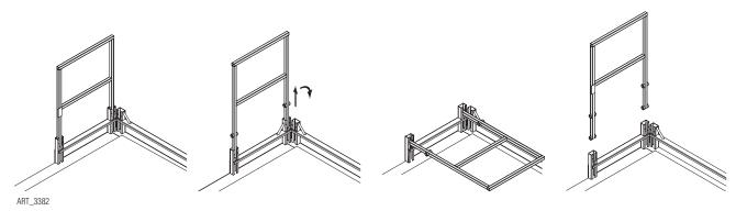
The TITAN Boom<sup>™</sup> uses a pinless guard rail system. After removing the loading gates, lift the guard rail section and pivot to stow, or lift further to remove the rail.
