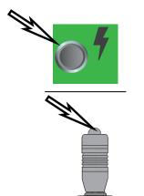
Lift functions (all boom, platform, chassis level and stabilizer operations) are enabled by pressing and holding the button on top of either the Boom or Platform control levers, or the green Enable button at the top left of the Platform Control Station. This allows the use of multiple boom and platform functions if desired.
