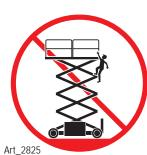
DO NOT fasten a fall restraint lanyard to an adjacent structure.
