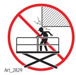
Watch for crushing hazards when holding the platform rail.
