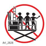
DO NOT exceed the maximum platform capacity (see Specifications). The weight of options and accessories will reduce the rated platform capacity and must be factored into the total platform load. Refer to the decals on the options.
