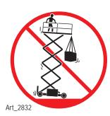
DO NOT attach overhanging loads or use the machine as a crane.
