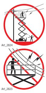
DO NOT work in close proximity to, or in contact with, energized power lines and electrical equipment. This machine is not insulated and WILL NOT protect the operator from injury or the machine from damage.
