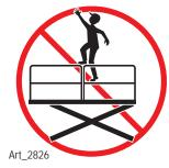
DO NOT sit, stand or climb on the platform guard rails. Maintain a firm footing on the platform floor at all times.
