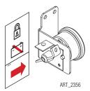
• Check Battery Disconnect Switch in Control Module next to Base Controls. Must be in ON position.
