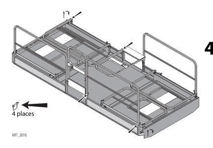
Remove the safety snap pins from main deck rail panels that attach to the entry gates.
