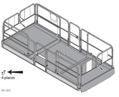
Remove the safety snap pins that secure the front and rear deck extension rail panels together. Lift the bracket connecting the tops of the deck extension rail panels.
