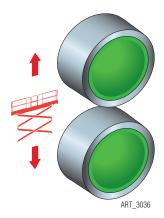
• Press and hold the RAISE button on the base control panel to elevate the platform.
