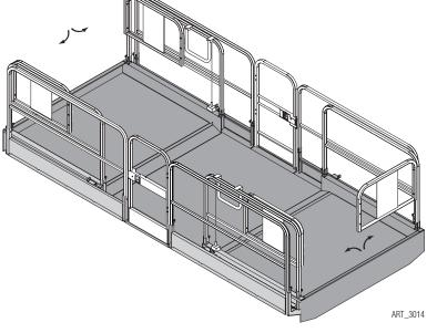
Remove the safety snap pins from the deck extension side rail bases.
