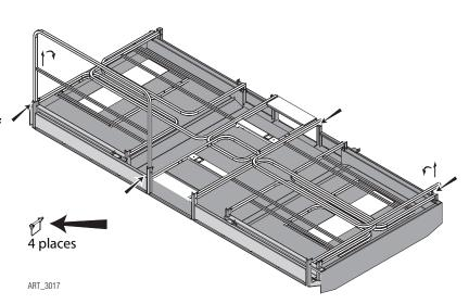
To return the machine to normal operation mode, lift all rails into their upright position, install all safety snap pins, and position the platform control box on the extension rail.
