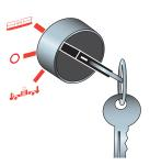
• Lower Control Box: Turn the Key Switch to PLATFORM.
