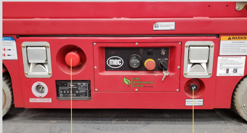
Emergency Battery Disconnect
