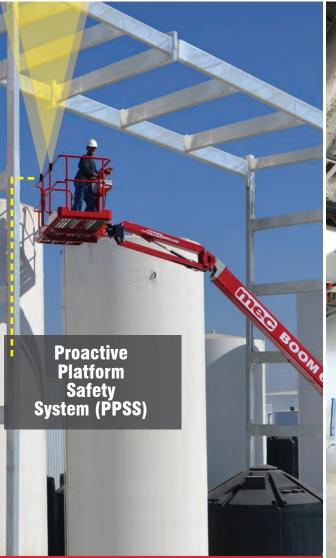
These safety innovations do not take the place of operator attentiveness. ALWAYS check over, under and around the machine for personnel, structures and obstructions before activating any control function and continue to watch for hazards while operating the machine.
