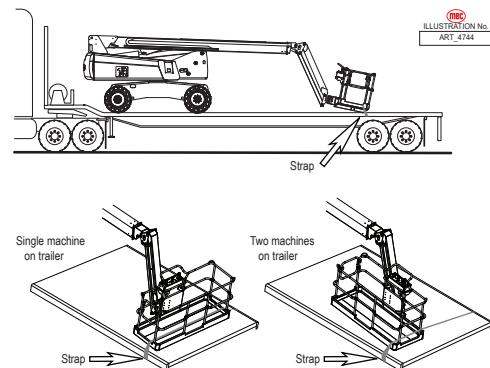
It may be necessary to turn the platform 90° when loading two machines on the same trailer. In this case, route the strap over the toeboard and through the end of the platform as shown.
