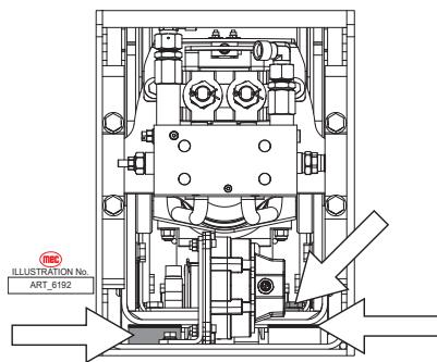
space between the sliding surface of the block and the sliding surface of the first boom exceeds 0.5mm, some pads will be need to be added. Tightens the bolts about with a torque of 73.7ft-lbs (100Nm).
