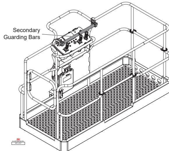
4. To enable limited operation while one or both bars are depressed, push up and hold the Emergency Platform Bypass switch (see illustration to right). While holding the Bypass switch, select the desired function and operate it in the normal procedure. Certain lift functions such as Riser Boom Up, Main Boom Up, and Telescope out are not available in this bypass mode.
