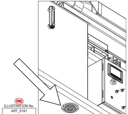
Park the machine and check the hydraulic oil level. If the oil level is low, add additional hydraulic fluid. Refer to page 22 for details on checking the hydraulic oil level.
