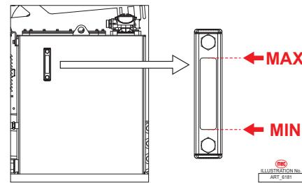
1. Make sure that the machine is parked on a flat, level surface.
