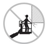
Check path before moving for crushing hazards when holding the platform rail.
