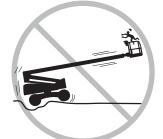
DO NOT DRIVE ON UNEVEN OR UNSTABLE SURFACE WHEN THE PLATFORM IS ELEVATED OR EXTENDED
