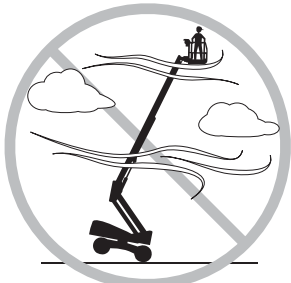
DO NOT ELEVATE IN GUSTY CONDITIONS OR WHEN WIND EXCEEDS 28 MPH (12.5 M/S)
