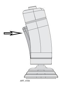
**Note:** If any Function Enable trigger or button is depressed for seven (7) seconds without any function being activated, the Enable System times out and deactivates. Release the trigger or button and reengage to activate the Function Enable System.
