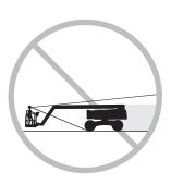
ALWAYS check over, under and around the machine for personnel, structures and obstructions before activating any control function and continue to watch for hazards while operating the machine.
