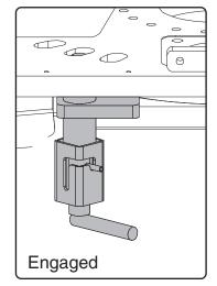
Before transport, rotate the turntable so that one of the three locking holes aligns with the Rotation Lock located on the chassis. The lock holes are located on the bottom of the Controls Module. The Rotation Lock is located on the chassis behind the left front wheel.
