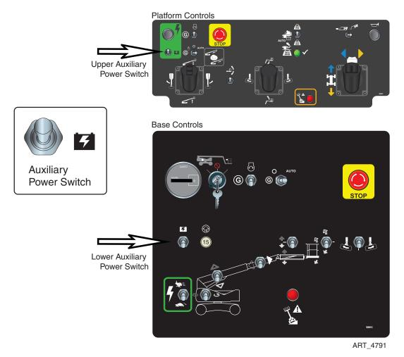
The Auxiliary Power System is used to lower the platform in case of primary power failure. To lower the platform, activate the Auxiliary Power Switch to run the auxiliary hydraulic pump.
