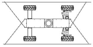
Make sure each of your chains is rated to hold the machine's weight (see serial number plate or Specifications). Use at least 4 chains.
