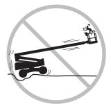
DO NOT DRIVE ON UNEVEN OR UNSTABLE SURFACE WHEN THE PLATFORM IS ELEVATED OR EXTENDED
