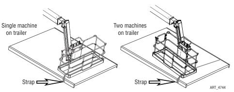
With the boom completely stowed, raise the jib slightly, then use the Platform Level function to lower the platform until the front of the platform touches the trailer surface.
