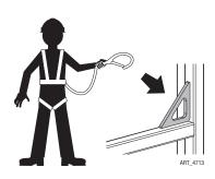
Personal fall protection equipment (PFPE) is required when operating this machine.
