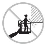
Check path before moving for crushing hazards when holding the platform rail.
