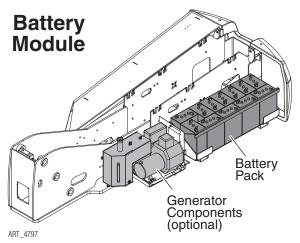
These instructions are for use with the optional Generator System. These components are located on the left side of the Batteries Module.
