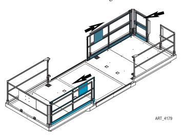
3 Use the Platform Slide function to slide the platform forward approximately 18 inches (46 cm). Use the ratcheting tie-down straps to secure the corners of the platform.
