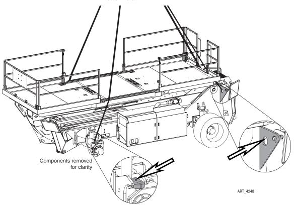
5 Locate the machine's center of gravity.
