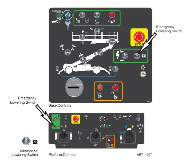
The Emergency Lowering System is used to lower the platform in case of power failure. To lower the platform, activate the Emergency Power Switch to run the Emergency Down auxiliary hydraulic pump.
