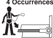
Personal fall protection equipment (PFPE) is required when operating this machine.
