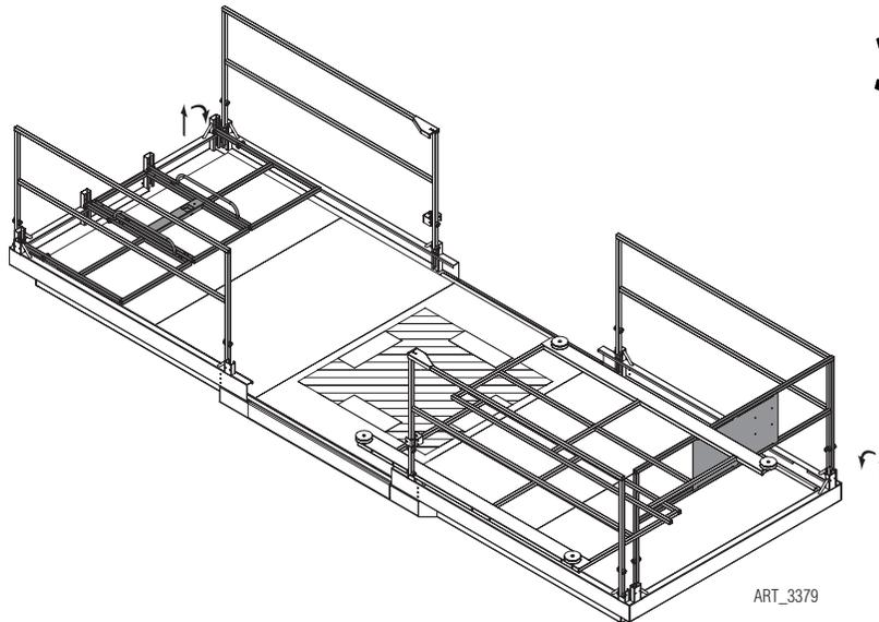
**3** Lift and pivot the end sections to the stowed position.
