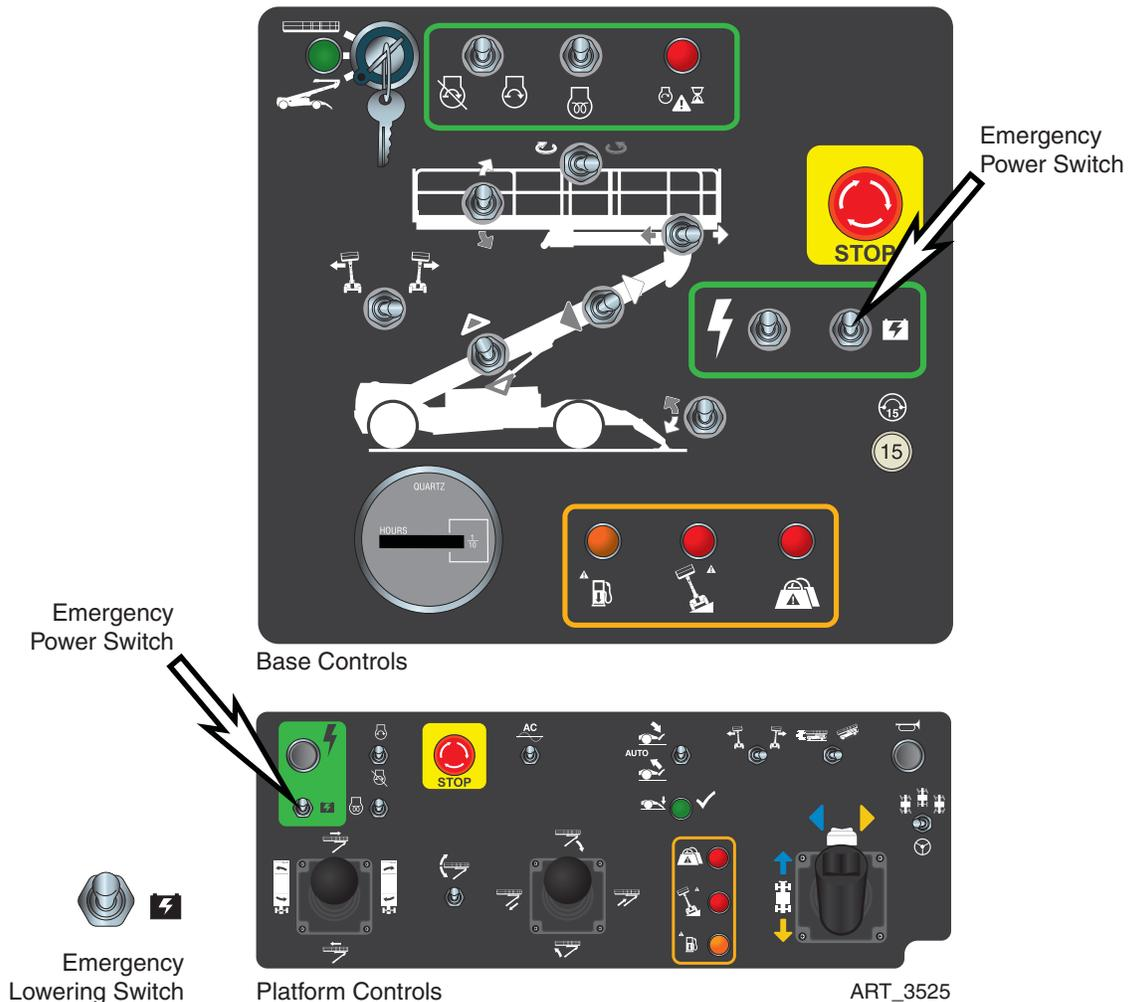
The Emergency Lowering System is used to lower the platform in case of power failure. To lower the platform, activate the Emergency Power Switch to run the Emergency Down auxiliary hydraulic pump.
