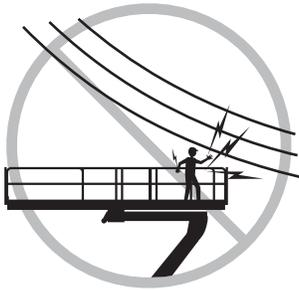
DO NOT work in close proximity to, or in contact with, energized power lines and electrical equipment. This machine is not insulated and WILL NOT protect the operator from injury or the machine from damage.
