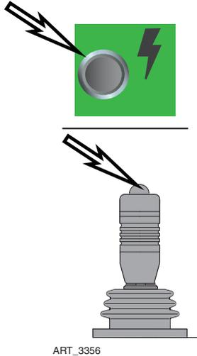
Lift functions (all boom, platform, chassis level and stabilizer operations) are enabled by pressing and holding the button on top of either the Boom or Platform control levers, or the green Enable button at the top left of the Platform Control Station. This allows the use of multiple boom and platform functions if desired.
