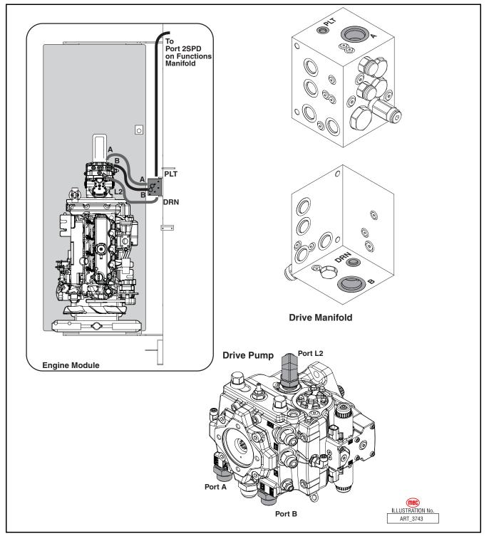
Figure 1-13: Drive Pump/Drive Manifold Connections
