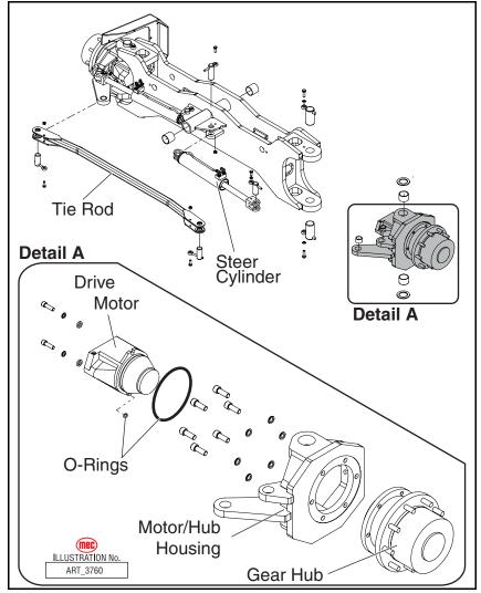
then remove the six bolts holding the gear hub to the motor/hub housing. Carefully remove the gear hub.
