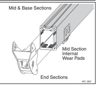
Mid Section Internal Wearpads as needed to achieve proper clearance.
