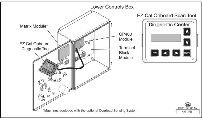
Figure 2-27: GP400 Control Module Location
