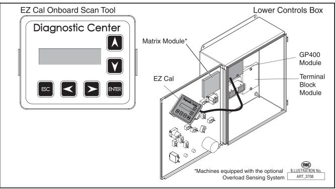
Figure 4-6: Onboard EZ-Cal Scan Tool & GP400 Module
