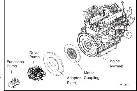
Figure 1-2: Engine & Hydraulic Pumps
