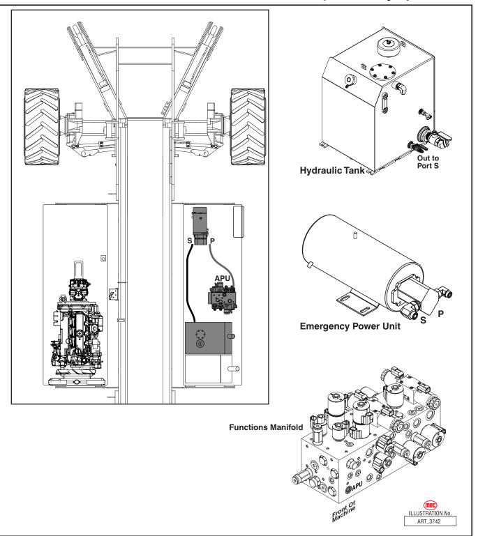
Figure 1-33: Emergency Power Circuit
