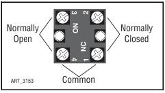
Figure 2-20: Toggle Switch, ON-OFF
