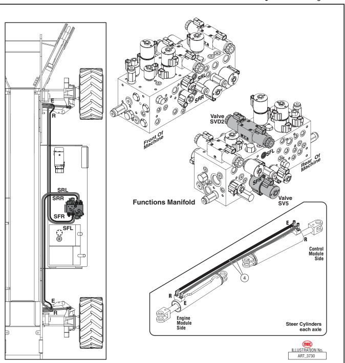
Figure 1-25: Steering Circuit
