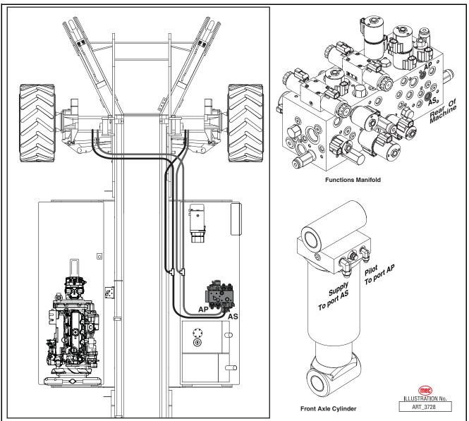
Figure 1-23: Axle Lock Cylinders
