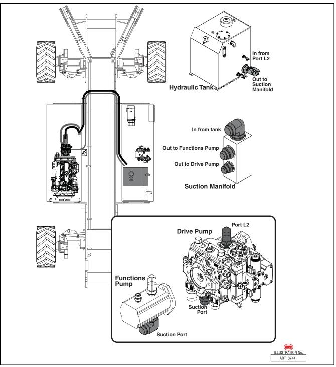
Figure 1-14: Drive Pump/Drive Manifold Connections
