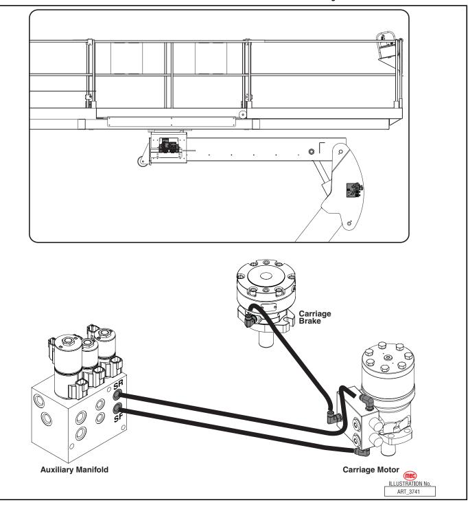
Figure 1-32: Platform Rotate Circuit
