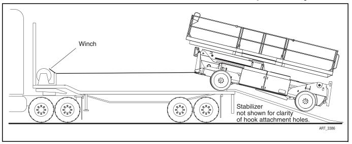
Figure 1-7: Loading the Machine
