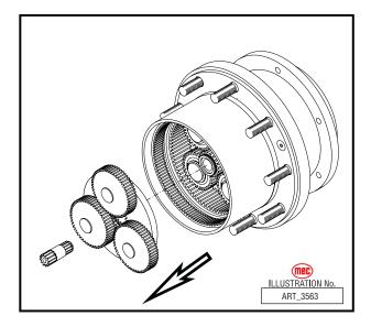
4. Remove the securing screws and remove the planetary ring.
