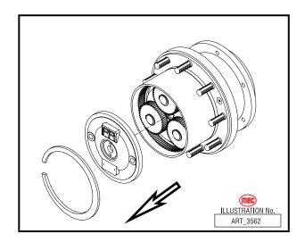
3. Pull out the pinion and the first stage reduction unit.
