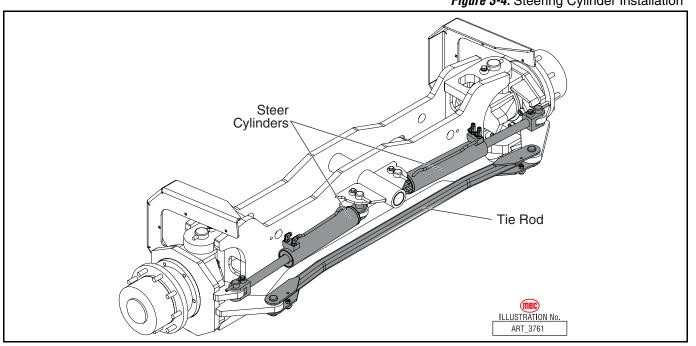
Figure 3-4: Steering Cylinder Installation
