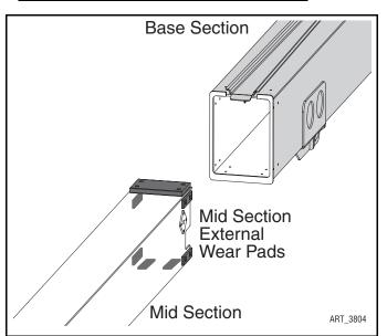
Introduction section of this manual for proper torque specifications. Insert the Mid Section into the Base Section of the boom.
