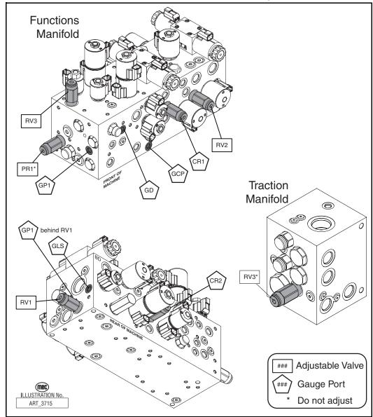
Figure 1-10: Adjustable Valves Location
