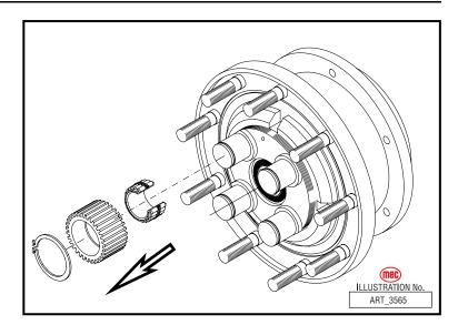
6. Unscrew the locking ring and remove the spindle from the hub support.
