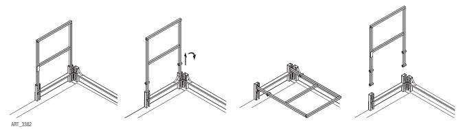
The TITAN Boom<sup>™</sup> uses a pinless guard rail system. After removing the loading gates, lift the guard rail section and pivot to stow, or lift further to remove the rail.
