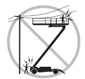
This machine **is not** electrically insulated and **will not** provide protection from contact with or proximity to electrical current.
