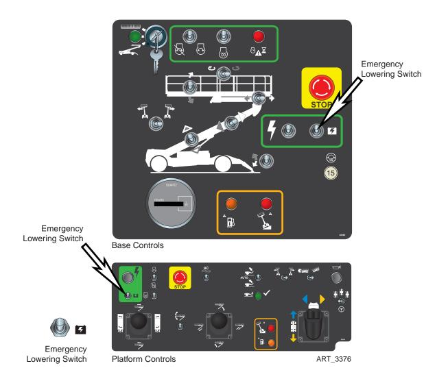
The Emergency Lowering System is used to lower the platform in case of power failure. To lower the platform, activate the Emergency Power Switch to run the Emergency Down auxiliary hydraulic pump.
