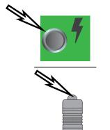
Lift functions (all boom, platform, chassis level and stabilizer operations) are enabled by pressing and holding the button on top of either the Boom or Platform control levers, or the green Enable button at the top left of the Platform Control Station. This allows the use of multiple boom and platform functions if desired.
