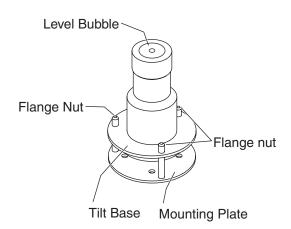
each corner is pressed. (There is approximately a three second delay). If the alarm does not sound, the flange nuts have been tightened too far. Loosen the nut on the 90° corners and repeat this test procedure.
