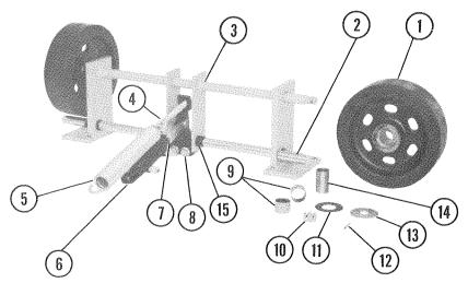
Figure 88. Rear Axle Assembly P.M. (215, 219)
