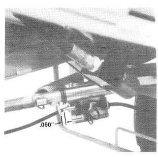
Figure 47. Stabilizer Switch Adjustment.
