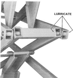
Figure 26. Scissors Lubrication.
