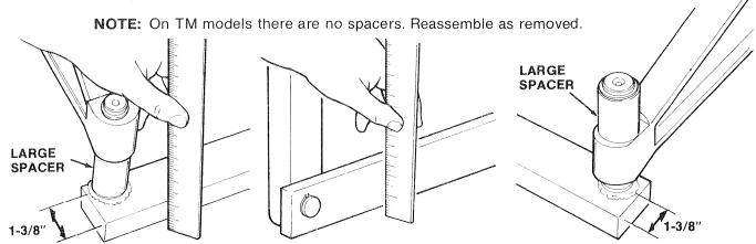
Figure 49. Stabilizer Bar Clearance Setting.
