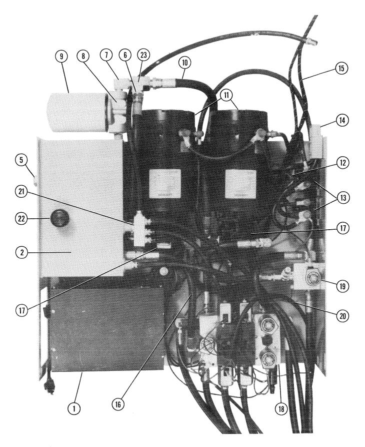
Figure 77. Component Tray Assembly (TM II & HT Shown)
