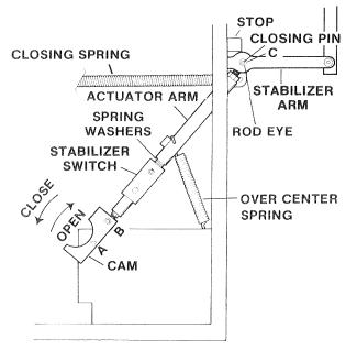
Figure 48. Activating Arm Adjustment.
