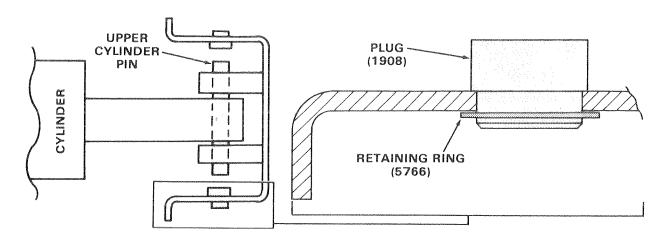
Figure 43. Top Cylinder Pin.
