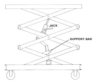
Figure 46. Installing Jack.
