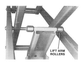
Figure 30. Lubricating Roller at Lift Arm.
