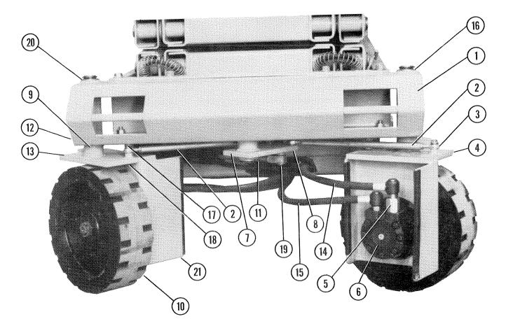
Figure 83. Front Drive Assembly, 2-Wheel Drive AM Models (216, 220)
