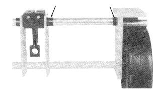
Figure 28. Lubricating Brake Linkage.
