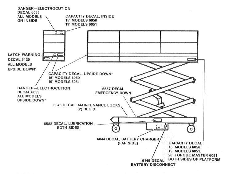
NOTE: Make sure capacity decals match capacity of machine.
