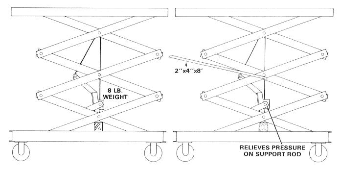
Figure 41. Counter Balancing Lift Arm.
