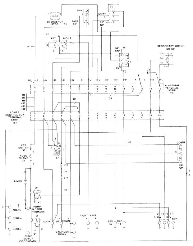
UP/DOWN SWITCH AT UPPER CONTROL BOX - CONTACTS MADE WITH TOGGLE AT KEYWAY POSITION 1-2, 4-5 — CENTER POSITION 1-2, 5-6 — OPPOSITE KEYWAY 2-3, 5-6 NOTE: F2 FUSE (2A) - EMERGENCY STOP, 1 USED: FORWARD, 2 USED: REVERSE, 2 USED.
