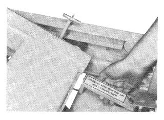
Figure 23. Positioning Maintenance Locks.
