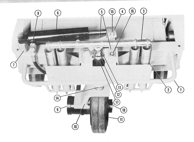
Figure 81. Front Drive Assembly, 1-Wheel Drive PM (115, 119)
