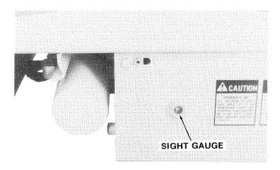
Figure 32. Hydraulic Oil Sight Gauge and Oil Filter.
