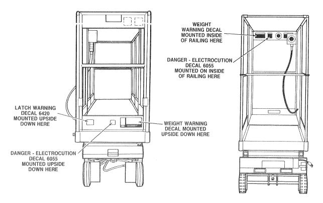
Figure 19. Warning Decal Installation.
