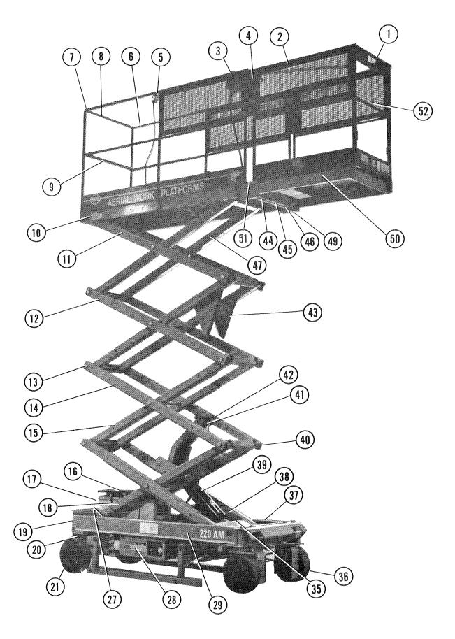
Figure 71. Models 216 AM (Not Shown) and 220 AM (Shown).
