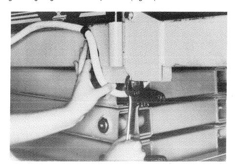
Figure 14. Leveling Platform.
