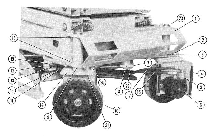
Figure 82. Front Drive Assembly, 2-Wheel Drive PM (215, 219)
