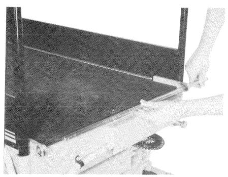
Figure 11. Pivot Pin Removal.
