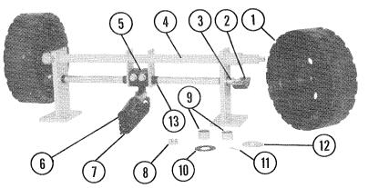
Figure 87. Rear Axle Assembly A.M. (216, 220)
