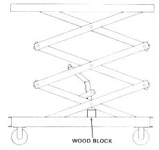
Figure 40. Installing Wood Block for Safety.
