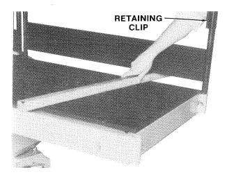
Figure 15. Right Hand Rail Installation.
