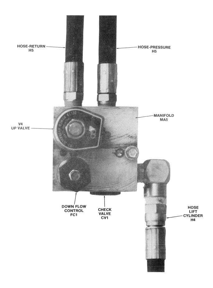
Figure 58. Manifold Assembly Battery Manual
