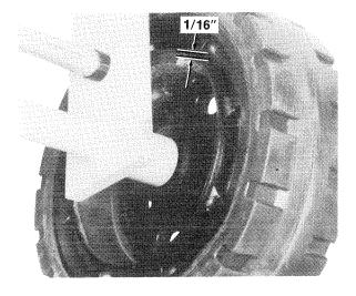
Figure 35. Brake Shoe Clearance.
