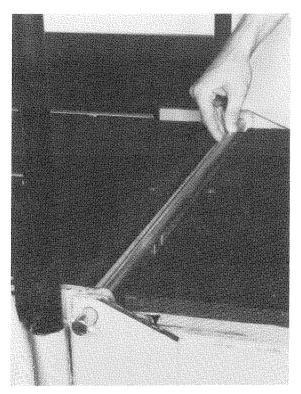
Figure 12. Pivot Pin Installation.
