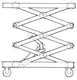
Figure 25. Scissors Lubrication Areas.
