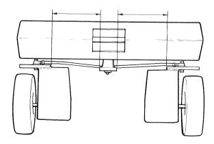
Figure 36. Aligning Front Wheels.
