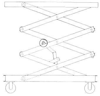
Figure 29. Lift Arm and Platform Lubrication Points.
