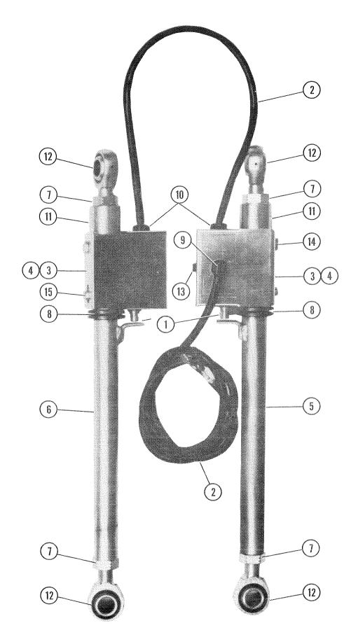
Figure 85. Stabilizer Activating arm Assembly - Part Number 2130
