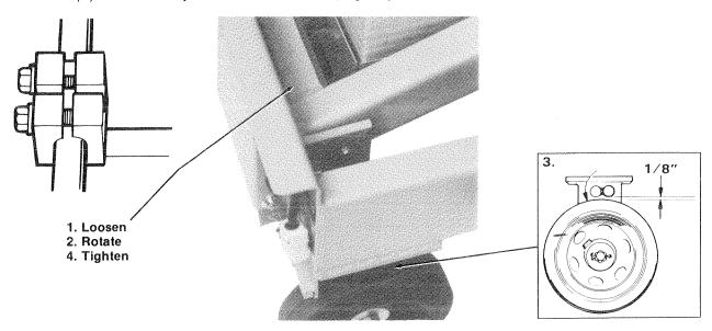
Figure 33. Adjusting Brakes.
