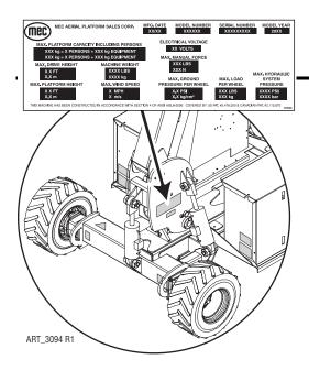
The serial plate is attached to the machine at the time of manufacture. Important information about the machine is recorded on the serial plate.
