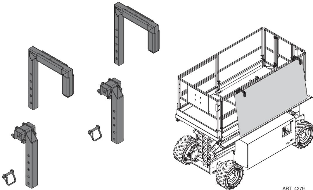
Remove the J-shaped arms from the Material Clamps when loading material on the Sheet Material Rack.
