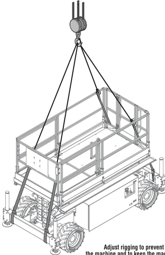
Adjust rigging to prevent damage to the machine and to keep the machine level.
