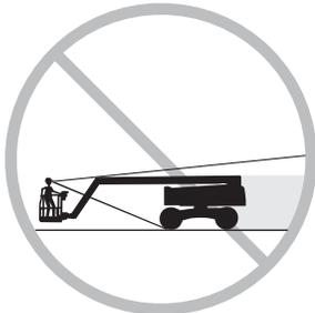
ALWAYS check over, under and around the machine for personnel, structures and obstructions before activating any control function and continue to watch for hazards while operating the machine.
